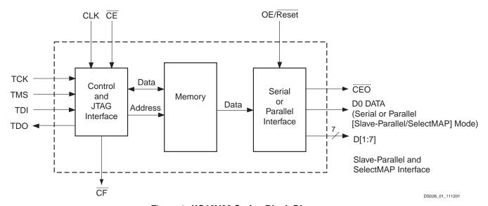
Figure 1: XC18V00 Series Block Diagram
