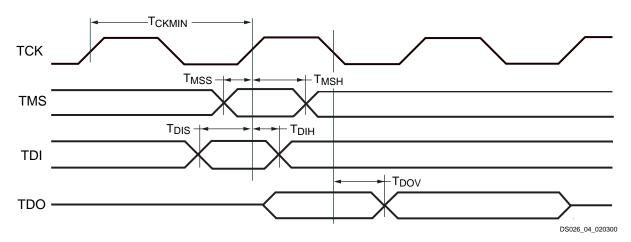
Figure 4: Test Access Port Timing
