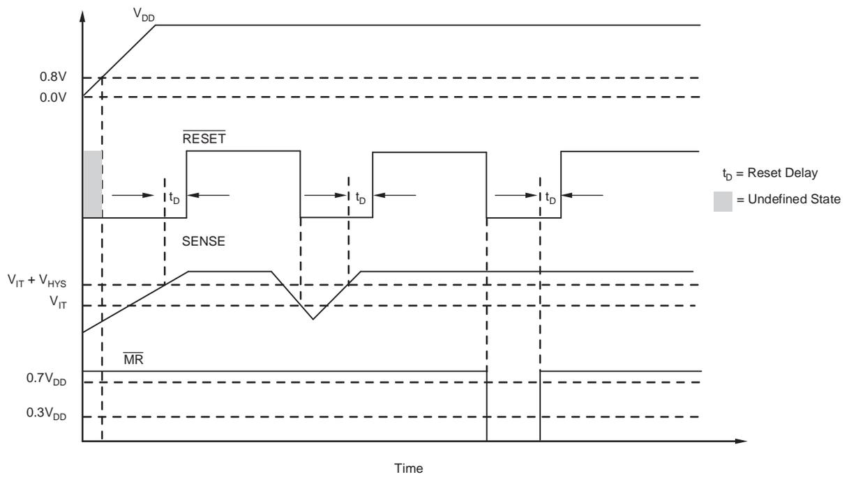
Figure 1.  $\overline{MR}$  and  $\overline{SENSE}$  Reset Timing Diagram
