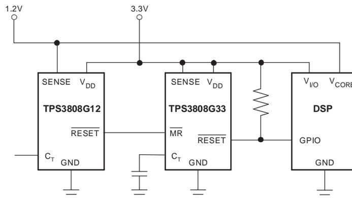
Figure 10. Using  $\overline{\text{MR}}$  to Monitor Multiple System Voltages
