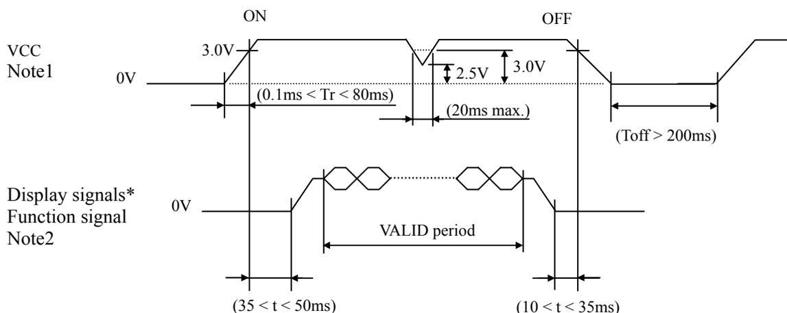
\* These signals should be measured at the terminal of 100Ω resistance.
