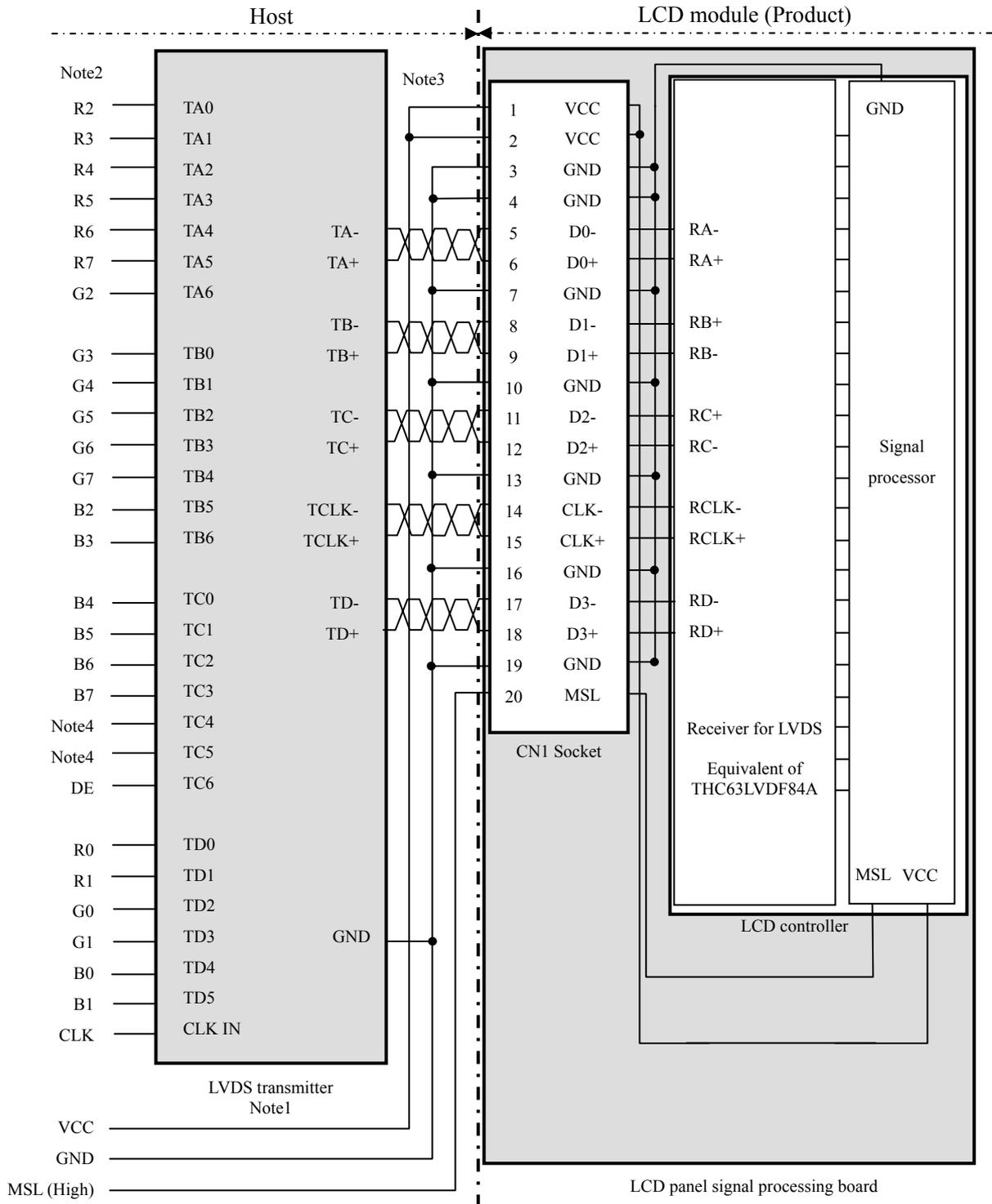
Note1: Recommended transmitter: THC63LVDF83A, THC63LVDM83R (Thine Electronics Inc.) or equivalent
