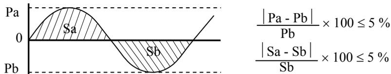
Pa: Supply voltage/current peak for positive, Pb: Supply voltage/current peak for negative
