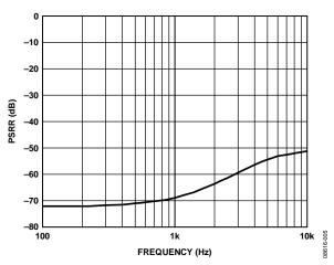
Figure 5. Typical Power Supply Rejection Ratio vs. Frequency
