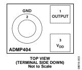
Figure 3. Pin Configuration
