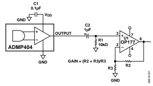
Figure 8. ADMP404 Connected to the OP177 Op Amp
