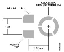
Figure 10. Suggested Solder Paste Stencil Pattern Layout
