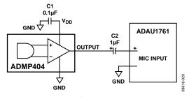
Figure 7. ADMP404 Connected to the Analog Devices ADAU1761 Codec
