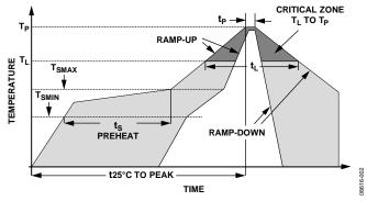
Figure 2. Recommended Soldering Profile Limits
