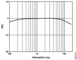
Figure 6. Typical Frequency Response (Measured)
