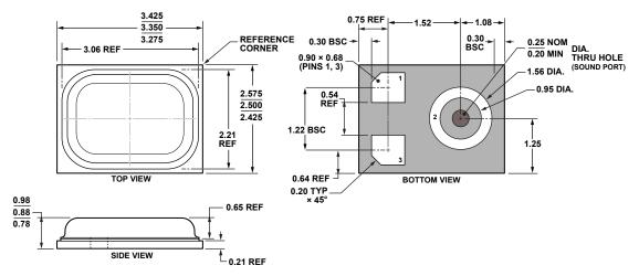
Figure 11. 3-Terminal Chip Array Small Outline No Lead Cavity [LGA\_CAV]
