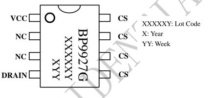
Figure 2. Pin configuration
