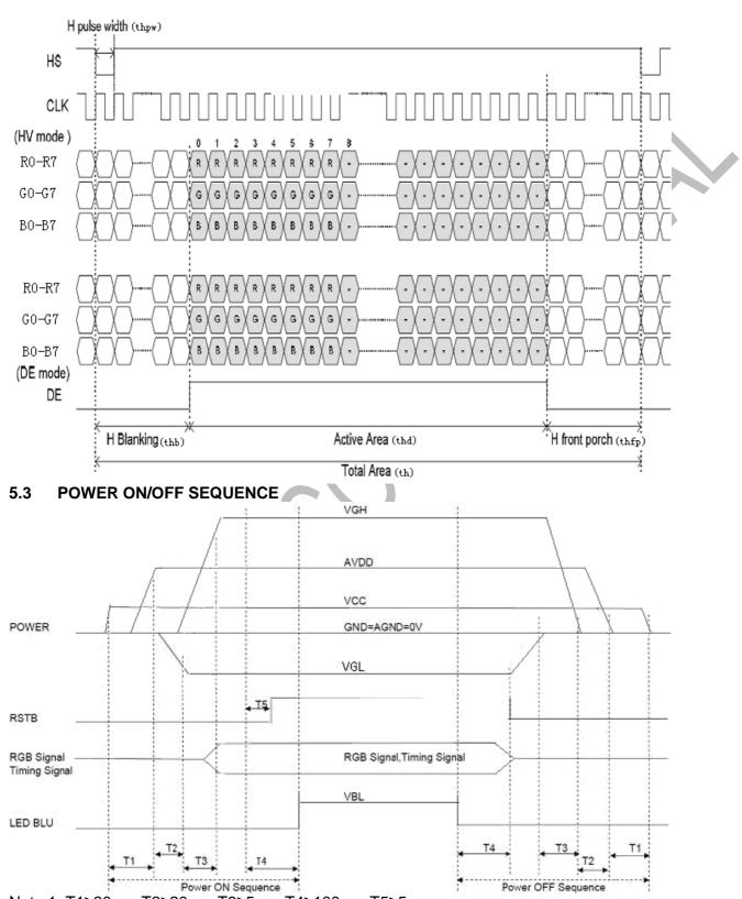
Note 1: T1≥20ms, T2≥20ms, T3≥5ms, T4≥100ms, T5≥5ms.
