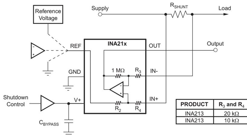
NOTE: 1-MΩ paths from shunt inputs to reference and INA21x outputs.
