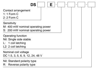
Note: 1 coil latching type are manufactured by lot upon receipt of order. Reverse polarity types available (add suffix-R)
