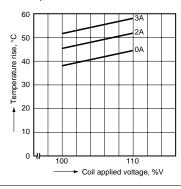
4-(2). Coil temperature rise (2 Form C 2 coil latching type) Tested sample: DS2E-ML2-DC12V Point measured: Inside the coil Ambient temperature: 20° to 21°C 68° to 70°F
