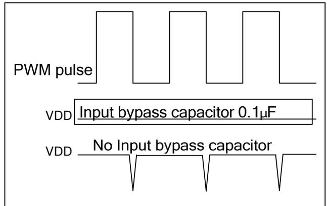
**Figure 3. Input Bypass Capacitor Affects the  $V_{DD}$  Drop.**
