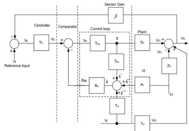
**Figure 4. Closed-Current Loop for Boost with PCM**
