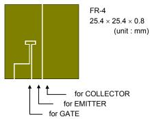
Note 2b : Device mounted on a glass-epoxy board (b)
