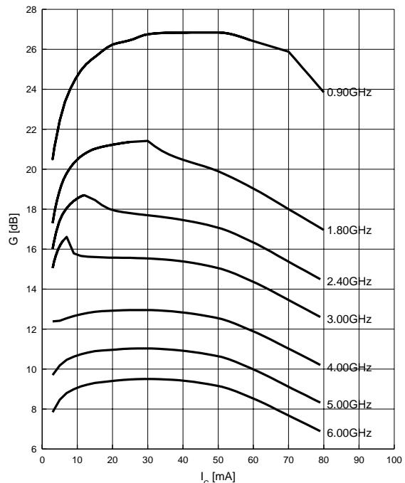
**Power gain  $G_{ma}, G_{ms} = f(V_{CE})$**
