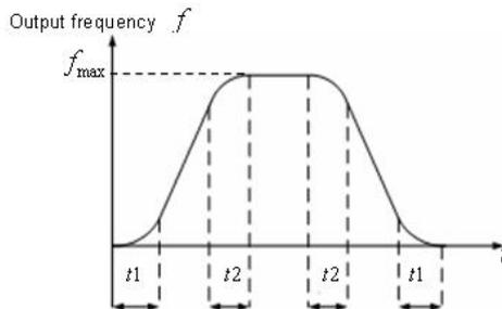
Figure 6.5 S curve diagram.
