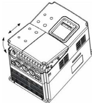
Figure 3.6 Disassembly of plastic cover.
