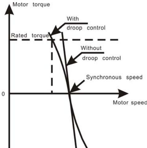
Figure 6.25 Droop control diagram
