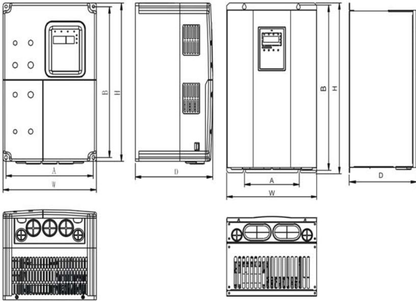
Figure1.4 Dimensions (15kW and below).
