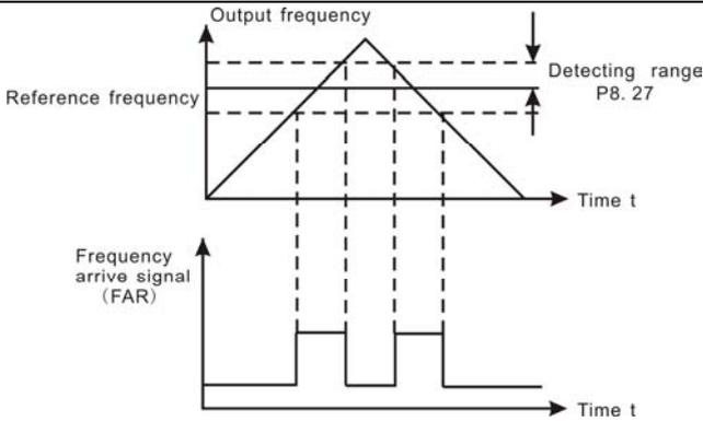
Figure 6.24 Frequency arriving detection diagram.
