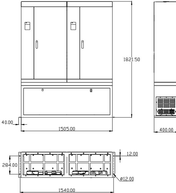
Figure 1.7 Dimensions (350kw~500W).
