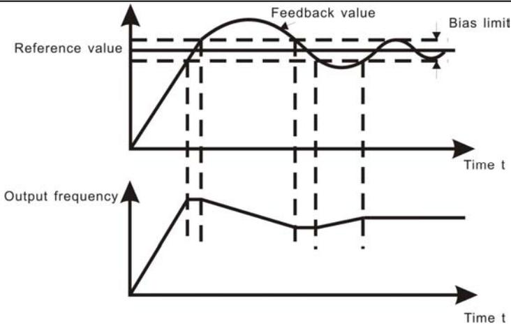
Figure 6.31 Relationship between bias limit and output frequency.
