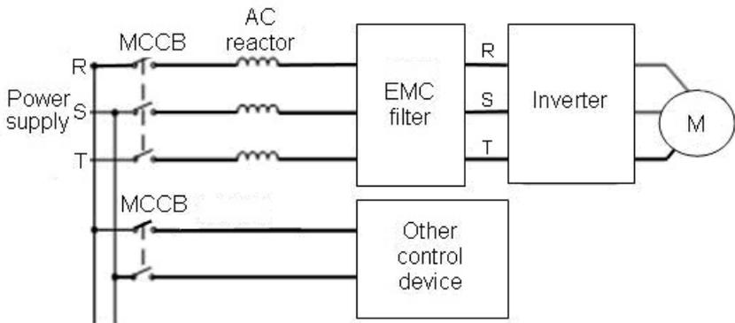
Figure4.9 Wiring at input side.
