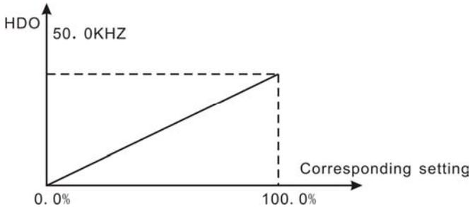
Figure 6.19 Relationship between HDO and corresponding setting.
