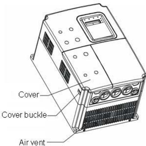
Figure 1.2 Parts of inverter (15kw and below).
