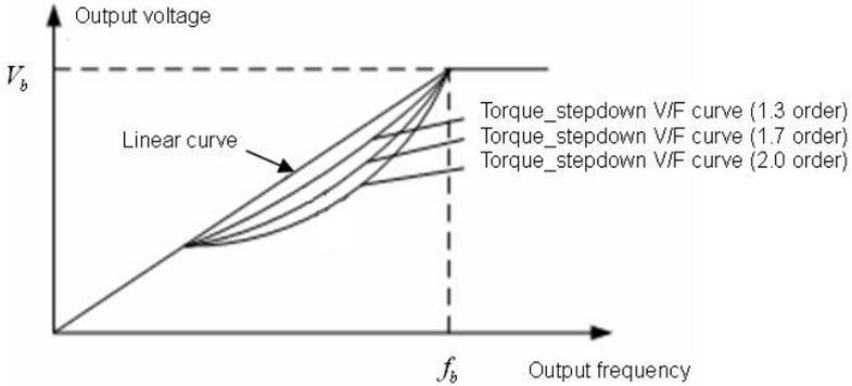
Figure 6.10 Multiple V/F curve diagram.
