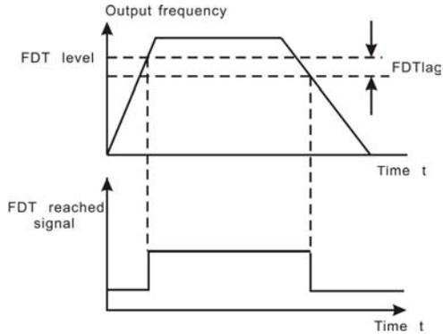
Figure 6.23 FDT Level diagram.
