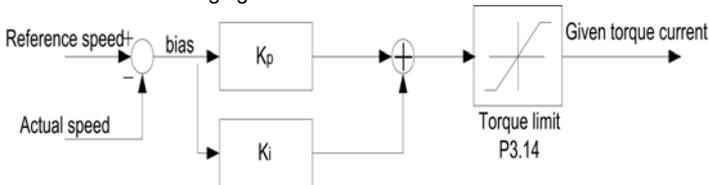
Figure 6.8 ASR diagram.
