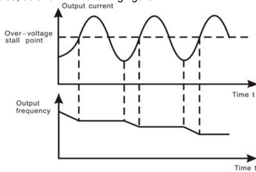
Figure 6.36 Over-voltage stall function.
