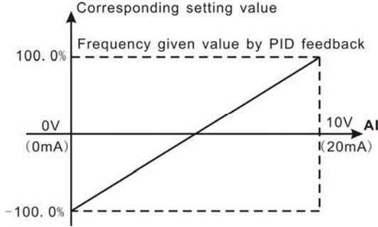
Figure 6.17 Relationship between AI and corresponding setting.
