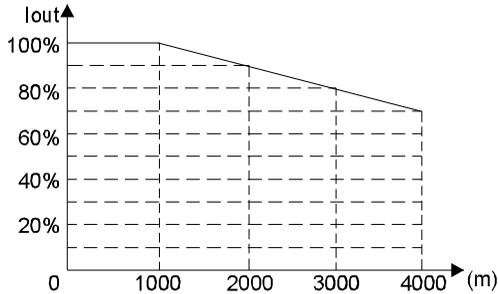
Figure 3.1 Relationship between output current and altitude.
