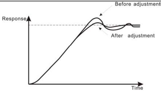
Figure 6.29 Reducing long-cycle oscillation diagram.
