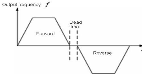
Figure 6.7 FWD/REV dead time diagram.
