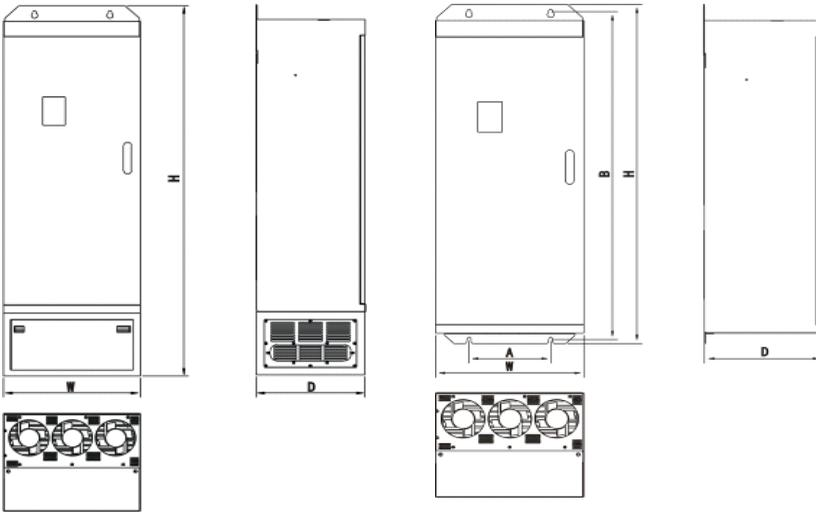
Figure 1.6 Dimensions (132~315kW).
