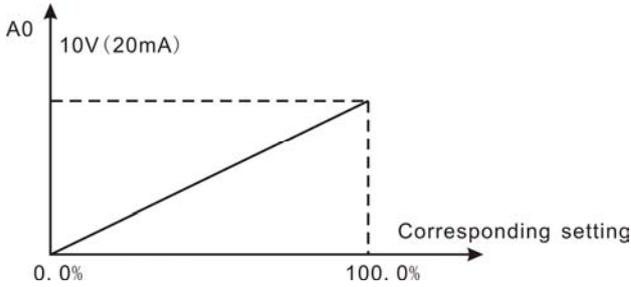
Figure 6.18 Relationship between AO and corresponding setting.
