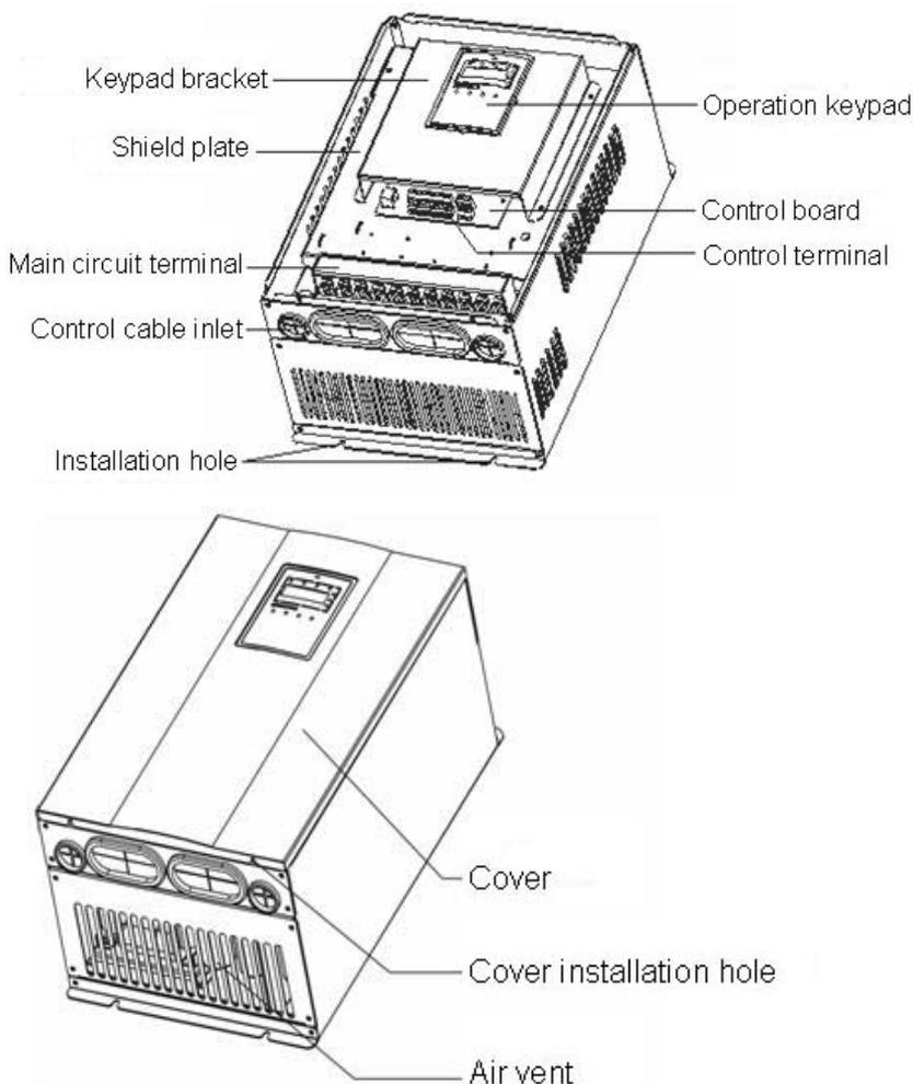
Figure 1.3 Parts of inverters (18.5KW and above).
