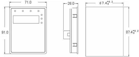
Figure 3.4 Dimensions of small keypad.
