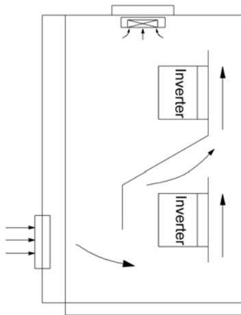
Figure 3.3 Installation of multiple inverters.
