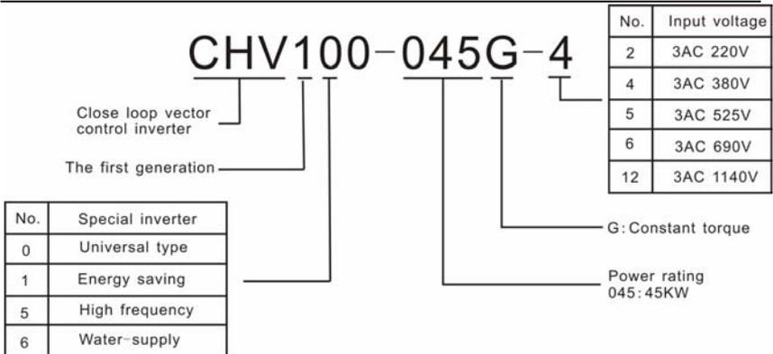
Figure 1.1 Nameplate of inverter.
