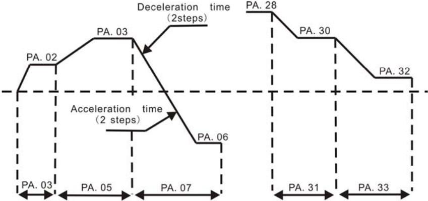
Figure 6.32 Simple PLC operation diagram.
