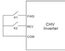
Figure 6.13 2-wire control mode 1.
