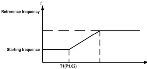
Figure 6.4 Starting diagram.
