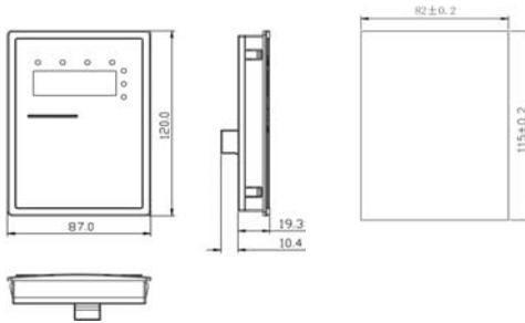
Figure 3.5 Dimensions of big keypad.
