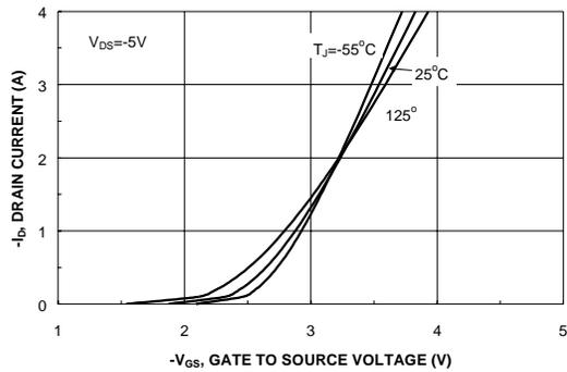
**Figure 5. Transfer Characteristics.**
