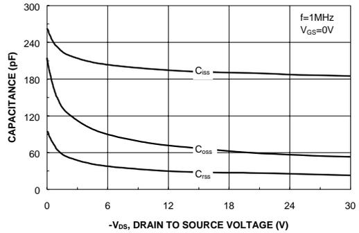
**Figure 8. Capacitance Characteristics.**
