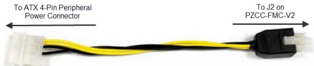
Figure 6 – ATX-to-6P Mini-Fit Adapter for Supplemental 12V PCIe Power
