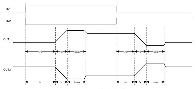
Figure 6. Propagation Delay Time
