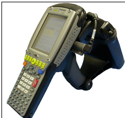
Figure B.2 RD7950 Installed On 7535 G2 Hand-Held Computer
