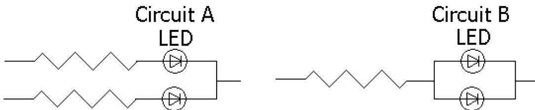
(a) Circuit A: it is recommended circuit.
