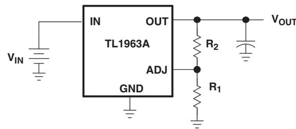
$$V_{OUT} = 1.21 \text{ V} \left( 1 + \frac{R_2}{R_1} \right) + (I_{ADJ})(R_2)$$
