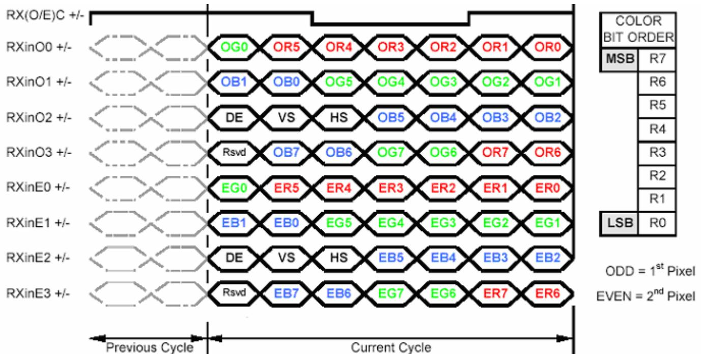
Note1: Normally DE mode only. VS and HS on EVEN channel are not used.
