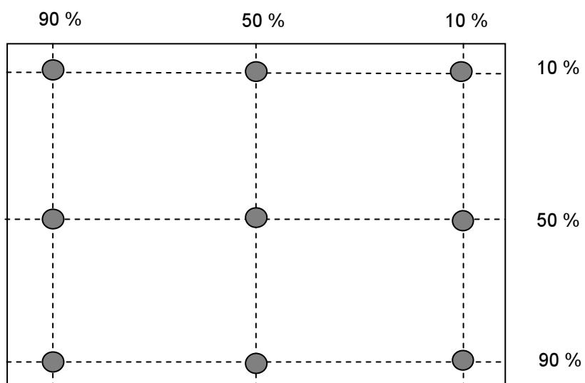
Note 3: The luminance uniformity of 9 points is defined by dividing the maximum luminance values by the minimum test point luminance. And measured by TOPCON SR-3
