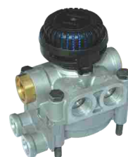
RELAY VALVE FYD NO.: FYD-85022 Original No.: 973 011 206 0 Ports: 1,21=M22x1.5 VOSS; 22,41,42=M16x1.5 VOSS WITH SILENCER
