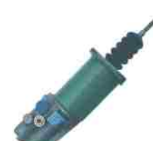
CLUTCH SERVO FYD NO.: FYD-61039 Original No.: VG3265 DIA: 75mm STROKE: 84mm AIR: M16 × 1.5 HYD: M14 × 1.5
