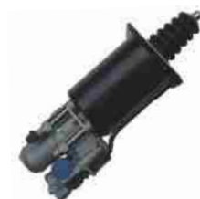
CLUTCH SERVO FYD NO.: FYD-61007 Original No.: 970 051 114 0 970 051 126 0 DIA: 76mm STROKE: 67mm AIR: M16 × 1.5 HYD: M14 × 1.5
