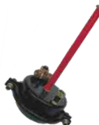
BRAKE CHAMBER FYD NO.: FYD-83011 TYPE: T20 STROKE: 57 PORT THREAD: M16×1.5 BOLT THREAD: M16×1.5 BOLT CENTRE: 120.7 PUSH ROD THREAD: M16×1.5 PUSH ROD LENGTH: Yourself
