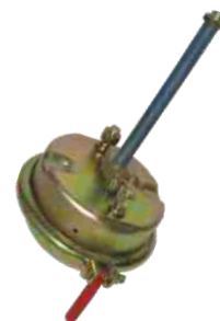
BRAKE CHAMBER FYD NO.: FYD-83007 TYPE: T24 STROKE: 57 PORT THREAD: 3/8"NPT BOLT THREAD: M16×1.5 BOLT CENTRE: 120.7 PUSH ROD THREAD: M16×1.5 PUSH ROD LENGTH: Yourself
