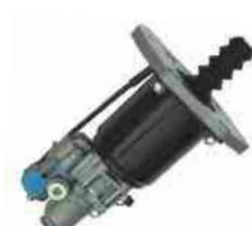
CLUTCH SERVO FYD NO.: FYD-61014 Original No.: 970 051 151 0 DIA: 85mm STROKE: 65mm AIR: M16 × 1.5 HYD: M14 × 1.5
