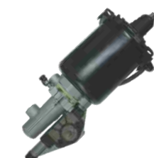
CLUTCH SERVO FYD NO.: FYD-61031 Original No.: 970 051 438 0 DIA: 102mm STROKE: 25.5mm AIR: M22 × 1.5 HYD: M14 × 1.5
