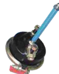
BRAKE CHAMBER FYD NO.: FYD-83013 TYPE: T20 STROKE: 57 PORT THREAD: M16×1.5 BOLT THREAD: M16×1.5 BOLT CENTRE: 120.7 PUSH ROD THREAD: M16×1.5 PUSH ROD LENGTH: Yourself
