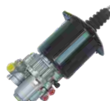
CLUTCH SERVO FYD NO.: FYD-61022 Original No.: 970 051 209 0 DIA: 102 mm STROKE: 26mm AIR: M16 × 1.5 HYD: M14 × 1.5
