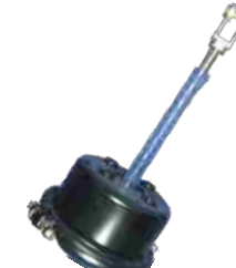
BRAKE CHAMBER FYD NO.: FYD-83020 TYPE: ZM443 STROKE: 64 PORT THREAD: 3/8"NPT BOLT THREAD: M12×1.5 BOLT CENTRE: PUSH ROD THREAD: M16×1.5 PUSH ROD LENGTH: Yourself
