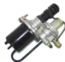
CLUTCH SERVO FYD NO.: FYD-61001 Original No.: 642-03080 DIA: 70mm STROKE: 35mm AIR: M14 × 1.5 HYD: M12 × 1.5
