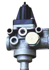
UNLOADER VALVE FYD NO.: FYD-86005 Original No.: 975 303 085 0 Cut Out Pressure: 9.5Bar Ports: 1+21=M22x1.5, 4+23=M12x1.5
