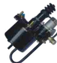
CLUTCH SERVO FYD NO.: FYD-61003 Original No.: 642-03505 DIA: 105mm STROKE: 35mm AIR: M14 × 1.5 HYD: M12 × 1.5
