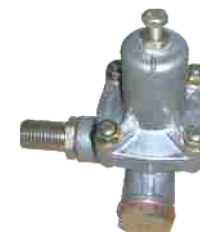
UNLOADER VALVE FYD NO.: FYD-86007 Original No.: 1054 Cut Out Pressure: 9.5Bar Ports: All Ports=M22x1.5
