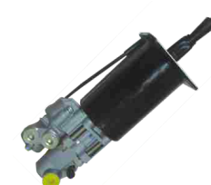
CLUTCH SERVO FYD NO.: FYD-61012 Original No.: 970 051 136 0 DIA: 75mm STROKE: 85mm AIR: M16 × 1.5 HYD: M14 × 1.5
