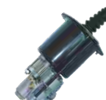
CLUTCH SERVO FYD NO.: FYD-61019 Original No.: 970 051 176 0 DIA: 102mm STROKE: 85mm AIR: M16 × 1.5 HYD: M14 × 1.5
