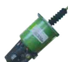
CLUTCH SERVO FYD NO.: FYD-61038 Original No.: VG3261 DIA: 102mm STROKE: 84mm AIR: M22 × 1.5 HYD: M14 × 1.5
