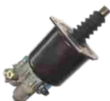
CLUTCH SERVO FYD NO.: FYD-61009 Original No.: 970 051 128 0 DIA: 102mm STROKE: 58.5mm AIR: M16 × 1.5 HYD: M14 × 1.5
