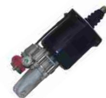
CLUTCH SERVO FYD NO.: FYD-61021 Original No.: 970 051 192 0 DIA: 100mm STROKE: 58.5mm AIR: M16 × 1.5 HYD: M14 × 1.5
