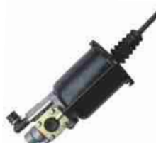
CLUTCH SERVO FYD NO.: FYD-61027 Original No.: 970 051 412 0 DIA: 102mm STROKE: 85mm AIR: M22 × 1.5 HYD: M14 × 1.5
