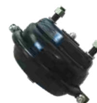
BRAKE CHAMBER FYD NO.: FYD-83009 TYPE: T24(DISC) STROKE: 57 PORT THREAD: M16×1.5 BOLT THREAD: M16×1.5 BOLT CENTRE: 120.7 PUSH ROD LENGTH: 15MM
