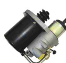
CLUTCH SERVO FYD NO.: FYD-61010 Original No.: 970 051 131 0 DIA: 85mm STROKE: 72mm AIR: M16 × 1.5 HYD: M14 × 1.5
