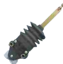
LEVELING VALVE FYD NO.: FYD-92001 Original No.: 464 007 011 0 Ports: 1,2=M10x1
