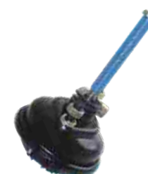
BRAKE CHAMBER FYD NO.: FYD-83017 TYPE: T16 STROKE: 57 PORT THREAD: M16×1.5 BOLT THREAD: M16×1.5 BOLT CENTRE: 120.7 PUSH ROD THREAD: M16×1.5 PUSH ROD LENGTH: Yourself
