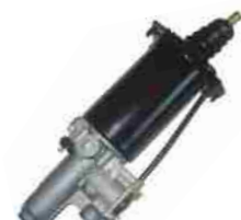
CLUTCH SERVO FYD NO.: FYD-61029 Original No.: 970 051 435 0 DIA: 75mm STROKE: 85mm AIR: M16 × 1.5 HYD: M14 × 1.5
