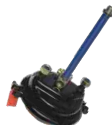
BRAKE CHAMBER FYD NO.: FYD-83008 TYPE: T24 STROKE: 64 PORT THREAD: 2-M16×1.5 BOLT THREAD: M16×1.5 BOLT CENTRE: 120.7 PUSH ROD THREAD: M16×1.5 PUSH ROD LENGTH: Yourself
