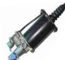
CLUTCH SERVO FYD NO.: FYD-61033 Original No.: 970 051 444 0 DIA: 75mm STROKE: 85mm AIR: M16 × 1.5 HYD: M14 × 1.5
