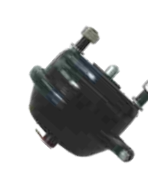
BRAKE CHAMBER FYD NO.: FYD-83018 TYPE: T16(DISC) STROKE: 57 PORT THREAD: 2-M16×1.5 BOLT THREAD: M16×1.5 BOLT CENTRE: 120.7 PUSH ROD LENGTH: 15mm
