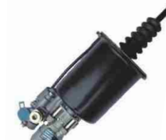
CLUTCH SERVO FYD NO.: FYD-61015 Original No.: 970 051 157 0 DIA: 102mm STROKE: 85mm AIR: M16 × 1.5 HYD: M14 × 1.5
