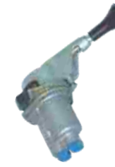
HAND BRAKE VALVE FYD NO.: FYD-88020 Original No.: 961 702 001 0 Ports: All Ports= M14x1.5
