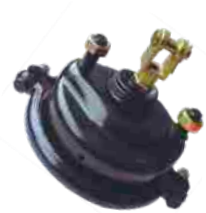
BRAKE CHAMBER FYD NO.: FYD-83010 TYPE: T24 STROKE: 57 PORT THREAD: M22×1.5 BOLT THREAD: M16×1.5 BOLT CENTRE: 120.7 PUSH ROD THREAD: M16×1.5 PUSH ROD LENGTH: Yourself
