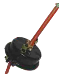
BRAKE CHAMBER FYD NO.: FYD-83006 TYPE: T24 STROKE: 64 PORT THREAD: 2-M16×1.5 BOLT THREAD: M16×1.5 BOLT CENTRE: 120.7 PUSH ROD THREAD: M16×1.5 PUSH ROD LENGTH: Yourself
