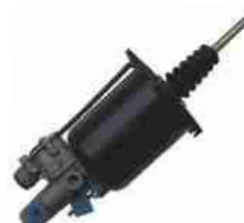
CLUTCH SERVO FYD NO.: FYD-61023 Original No.: 970 051 307 0 DIA: 102mm STROKE: 85mm AIR: M22 × 1.5 VOSS HYD: M14 × 1.5
