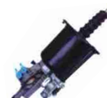
CLUTCH SERVO FYD NO.: FYD-61034 Original No.: 970 051 455 0 DIA: 102mm STROKE: 25.2mm AIR: M16 × 1.5 HYD: M14 × 1.5
