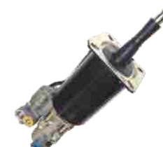
CLUTCH SERVO FYD NO.: FYD-61011 Original No.: 970 051 132 0 DIA: 105mm STROKE: 85mm AIR: M16 × 1.5 HYD: M14 × 1.5
