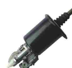
CLUTCH SERVO FYD NO.: FYD-61018 Original No.: 970 051 164 0 DIA: 102mm STROKE: 85mm AIR: M16 × 1.5 HYD: M14 × 1.5
