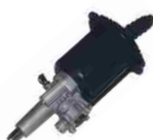
CLUTCH SERVO FYD NO.: FYD-61030 Original No.: 970 051 436 0 DIA: 102mm STROKE: 85mm AIR: M16 × 1.5 HYD: M14 × 1.5
