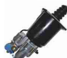
CLUTCH SERVO FYD NO.: FYD-61020 Original No.: 970 051 190 0 DIA: 85mm STROKE: 65mm AIR: M16 × 1.5 HYD: M14 × 1.5
