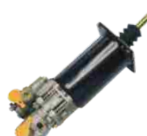
CLUTCH SERVO FYD NO.: FYD-61006 Original No.: 970 051 111 0 DIA: 75mm STROKE: 85mm AIR: M16 × 1.5 HYD: M14 × 1.5
