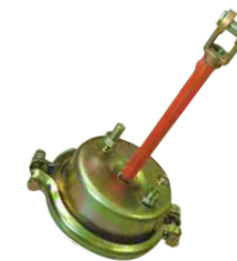
BRAKE CHAMBER FYD NO.: FYD-83016 TYPE: T16 STROKE: 57 PORT THREAD: 2-3/8"NPT BOLT THREAD: M12×1.5 BOLT CENTRE: 76 PUSH ROD THREAD: M14×1.5 PUSH ROD LENGTH: Yourself
