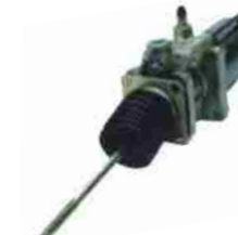
CLUTCH SERVO FYD NO.: FYD-61054 Original No.: APGA1610/4 DIA: 75mm STROKE: 67mm AIR: M16 × 1.5 HYD:
