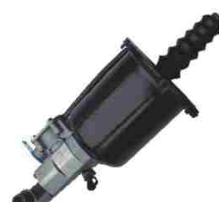
CLUTCH SERVO FYD NO.: FYD-61028 Original No.: 970 051 431 0 970 051 405 0 DIA: 102 mm STROKE: 85mm AIR: M16 × 1.5 HYD: M14 × 1.5
