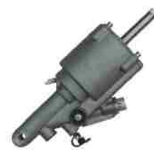
CLUTCH SERVO FYD NO.: FYD-61042 Original No.: 626639AM DIA: 95mm STROKE: 70mm AIR: M16 × 1.5 HYD: M14 × 1.5
