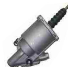
CLUTCH SERVO FYD NO.: FYD-61045 Original No.: 625586AM DIA: 100mm STROKE: 85mm AIR: M16 × 1.5 HYD: M14 × 1.5
