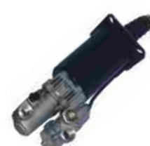
CLUTCH SERVO FYD NO.: FYD-61013 Original No.: 970 051 137 0 DIA: 75mm STROKE: 85mm AIR: M16 × 1.5 HYD: M14 × 1.5
