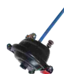
BRAKE CHAMBER FYD NO.: FYD-83019 TYPE: T12 STROKE: 57 PORT THREAD: 3/8"NPT BOLT THREAD: M12×1.5 BOLT CENTRE: 76 PUSH ROD THREAD: M14×1.5 PUSH ROD LENGTH: Yourself
