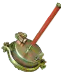
BRAKE CHAMBER FYD NO.: FYD-83012 TYPE: T20 STROKE: 57 PORT THREAD: 2-M16×1.5 BOLT THREAD: M16×1.5 BOLT CENTRE: 120.7 PUSH ROD THREAD: M16×1.5 PUSH ROD LENGTH: Yourself
