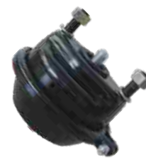
BRAKE CHAMBER FYD NO.: FYD-83014 TYPE: T20(DISC) STROKE: 57 PORT THREAD: 2-M16×1.5 BOLT THREAD: M16×1.5 BOLT CENTRE: 120.7 PUSH ROD LENGTH: Yourself
