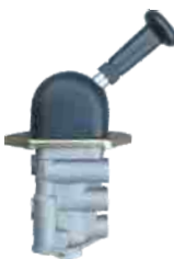
HAND BRAKE VALVE FYD NO.: FYD-88005 Original No.: 961 722 258 0 Ports: 5-M22x1.5 VOSS Ports: 11,21,22=M14x1.5
