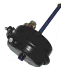
BRAKE CHAMBER FYD NO.: FYD-83005 TYPE: T30 STROKE: 64 PORT THREAD: 2-M16×1.5 BOLT THREAD: M16×1.5 BOLT CENTRE: 120.7 PUSH ROD THREAD: M16×1.5 PUSH ROD LENGTH: Yourself
