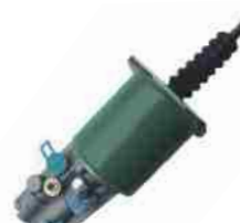
CLUTCH SERVO FYD NO.: FYD-61037 Original No.: VG3208 DIA: 100mm STROKE: 84mm AIR: M16 × 1.5 HYD: M14 × 1.5
