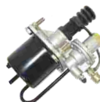
CLUTCH SERVO FYD NO.: FYD-61002 Original No.: 642-03502 DIA: 90mm STROKE: 35mm AIR: M14 × 1.5 HYD: M12 × 1.5
