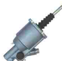
CLUTCH SERVO FYD NO.: FYD-61046 Original No.: 628493AM 628494AM DIA: 100mm STROKE: 85mm AIR: M16 × 1.5 HYD: M14 × 1.5
