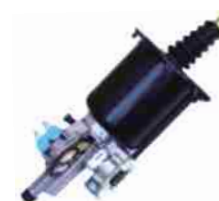
CLUTCH SERVO FYD NO.: FYD-61024 Original No.: 970 051 402 0 DIA: 102mm STROKE: 25.2mm AIR: M16 × 1.5 HYD: M14 × 1.5
