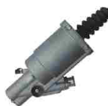
CLUTCH SERVO FYD NO.: FYD-61044 Original No.: 628276AM DIA: 80mm STROKE: 85mm AIR: M16 × 1.5 HYD: M14 × 1.5
