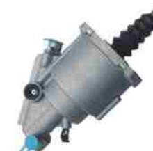
CLUTCH SERVO FYD NO.: FYD-61047 Original No.: 622190AM 622108AM DIA: 100mm STROKE: 70mm AIR: M16 × 1.5 HYD: M14 × 1.5
