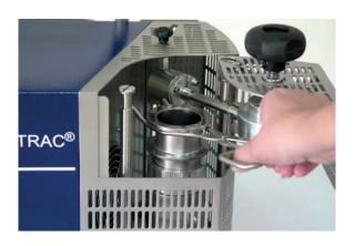
and mg water content. Other volatile substances are condensed in a cooling trap at room temperature and therefore do not participate in the measurement. It is therefore an absolute measurement method exclusively for water - as also described in DIN EN ISO 15512:2019 as method E - Determination of water content by the calcium hydride method.
