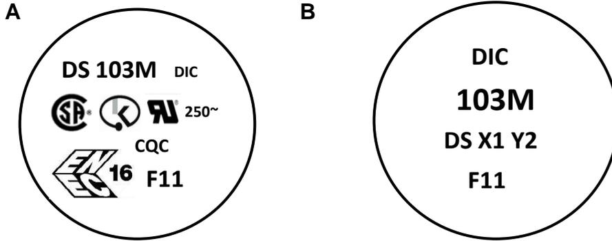
\* Safety certifications can be printed on either the capacitor body or packing label.
