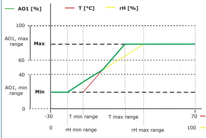
**Note:** The output changes automatically depending on the higher of the T and rH values, i.e. the higher of two output values controls the output. See the green line in the operational diagram above.
