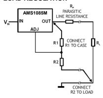
True remote load sensing it is not possible to provide, because the AMS1085M is a three terminal device. The resistance of the wire connecting the regulator to the load will limit the load regulation.
