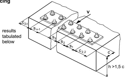
Note: It is assumed that only the row of anchors closest to the free concrete edge carries the centric shear load
