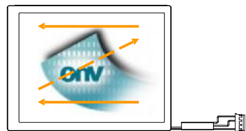
Fig. 2 Reverse scan (Pin4, DPS = High)
