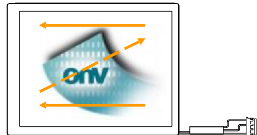
Fig. 2 Reverse scan (Pin4, DPS = High)
