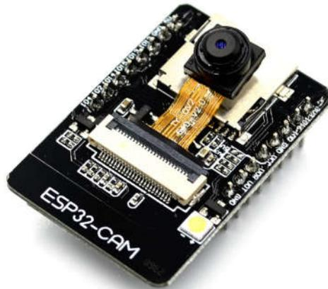
This development board is an ESP32 based board with WiFi and Bluetooth and has a built-in camera. In addition, the board also has a micro SD card connection.
